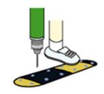
Drill 12MM diameter holes into the surface, through the existing holes of the placed units. The holes should be 120-140MM deep in order to accommodate the plastic shields that are 100MM long.
