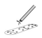
Make sure the holes are clear of dust and debris before installing the shields. After each hole is drilled, insert a plastic shield in order to keep the units from shifting.
